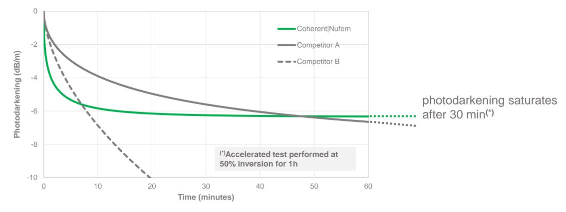
Photodarkening saturates two times faster than competition ensuring reliable operation and extended lifetime
